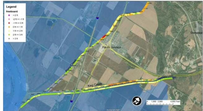
Figure 3.3-17. Estimated freeboard along Pony and Keg creeks near Pacific Junction, Iowa. No overtopping allowed.
