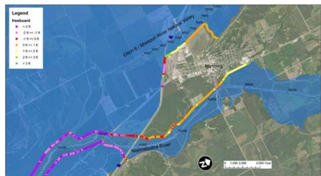
Figure 3.3-10. Estimated freeboard along Nishnabotna River near Hamburg, Iowa. No overtopping allowed.
