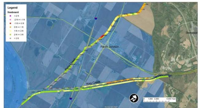
Figure 3.3-18. Depiction of inundation behind the levees if Keg Creek is overtopped at lowest freeboard location.
