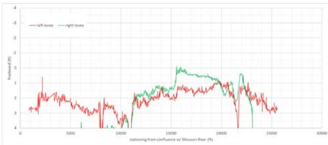
Figure 3.3-21. Estimated freeboard along Keg Creek for the left and right levees.
